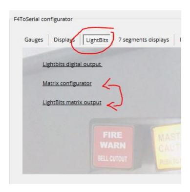
There are 3 links in this topic. The first link "LightBits Digital output" is used to connect the LEDS directly on the card. The other two are used to create and configure a matrix.
