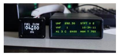
F4ToSerial allows obtaining the same level of result, except the scrolling effect of the numbers on the FFI. I would surely develop an update on this.
